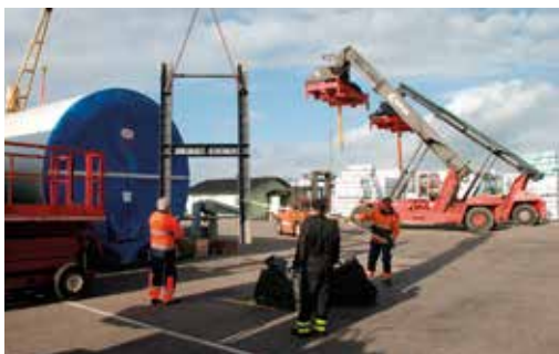
Customised services performed. The tower sections being prepared for transportation by dismantling frames
